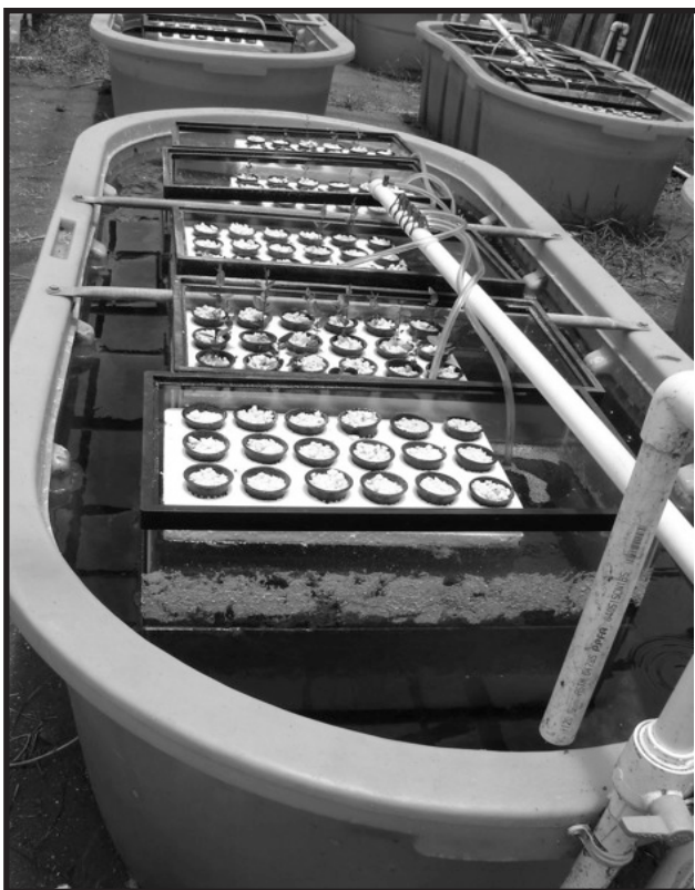
Figure 4. A block in the actual experiment. Each block consisted of a 300-gallon tank that held five glass aquaria for temperature control. Each of the five treatments was represented once per block.
