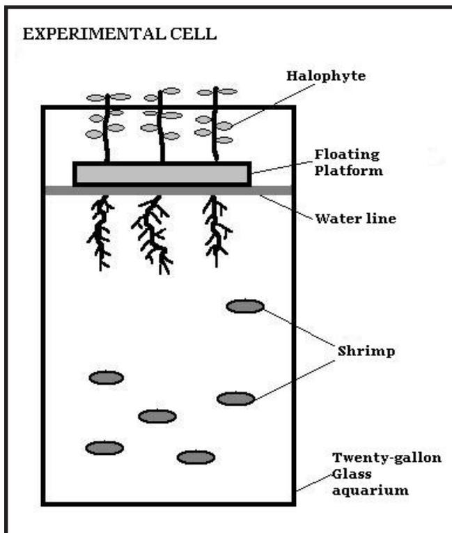
**Figure 3.** Cultivating saltwater plants and shrimp in the same space. Plants were grown in a floating platform that sits on top of the water. Roots were allowed to extend into the water. The only nutrient input to the system was shrimp feed.
