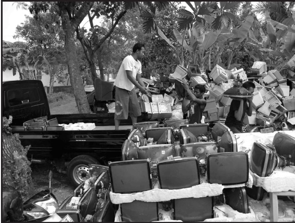
**Figure 1.** The collection and manual dismantling of CRT Monitors waste in Yogyakarta, Indonesia.
